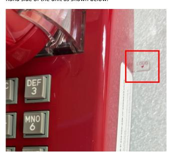
The ringer volume can be adjusted while the **HON-AOR-SCU-1 Sub-Command Unit** is mounted to the wall—move the lever up to decrease the volume, move the lever down to increase the volume.
